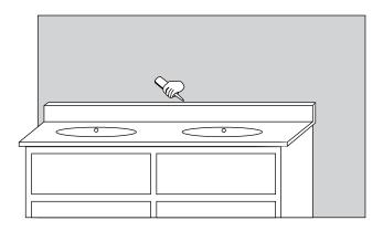
4. Let the assembled vanity sit for 24 hours to allow all the silicone sealant to fully dry. Once dry, proceed to the installation of your faucet and drain.
