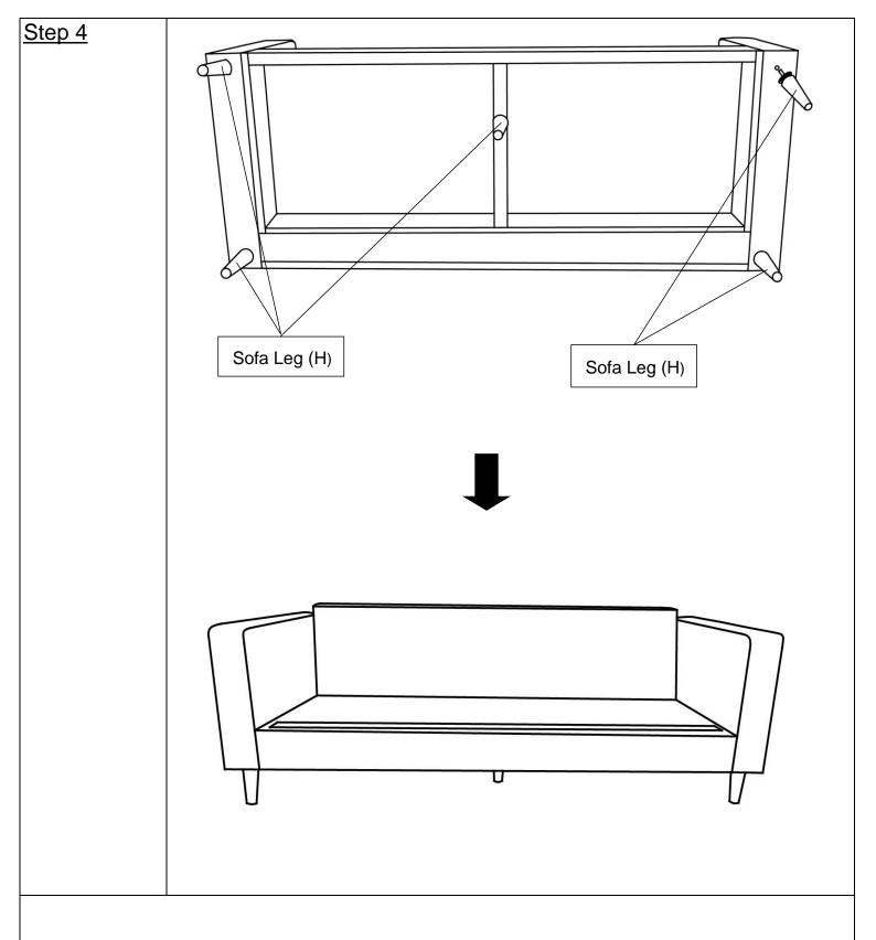
Install one of the Sofa Legs(H) at the bottom of the sofa by placing one Gasket(③) on the threaded stem. Then insert the threaded stem into the threaded mounting postion at the corner of the Sofa.
