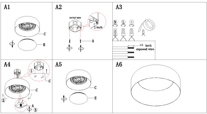
Step A1 » Unscrew lampshade (E) from fixture body (C).
