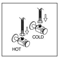
5. Attach flexible hose to water supply.
