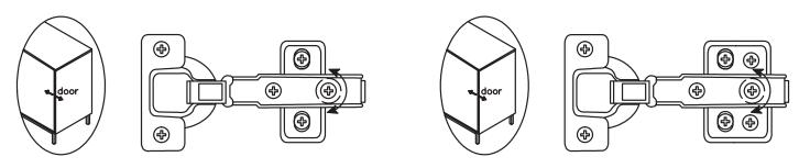
Adjust the in-and-out screws until the door is aligned with the side of the cabinet.
