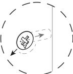
Still having issues? If a cam lock seems to be spinning in place or is not "catching" or pulling the panels together as expected, first remove the cam lock & try again while making sure that everything is properly positioned & oriented.
