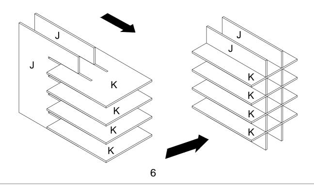
Step 8. Slide assembled unit (parts J & K) into place.
