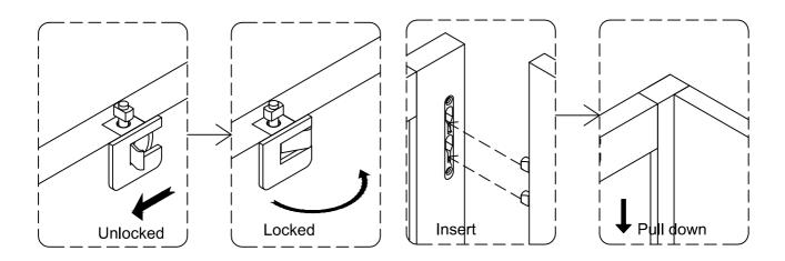
Reference the images above any time the instructions state "lock the hardware" or "insert hardware and pull down to lock".
