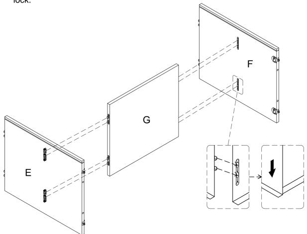
Step 3. Attach panels (parts B & C) and assembled unit (parts E, F & G) to bottom panel (part D) pull down to lock.
