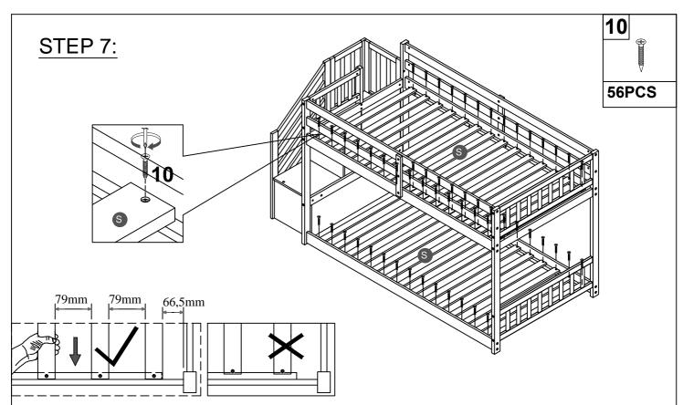
Note: Do not lock the screws of the bed slats to the outermost edge of the bed slats, you need to leave a certain space at the edges, otherwise it will cause the board to break. Do not lock the bed slats on the edge of the wood, please hold firmly before screwing, hold it in place with one hand, then lock the screw.
