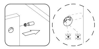
Next, you will notice the cam lock has a "C" shaped back. Commonly, an arrow on the front of the cam lock points in the same direction as the open section on back.
