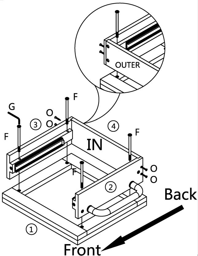
The above drawing is shown with the table top upside down - parts 2 & 3 must have the slides oriented with the open side closest to the front of the cart and the push bar on the left side of the cart as you look at it.
