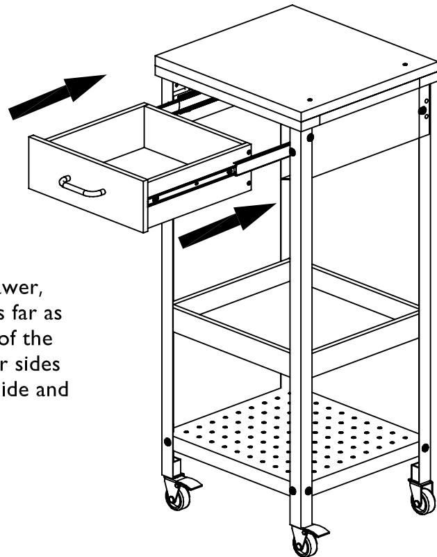
Before inserting the assembled drawer, please pull the drawer glides out as far as they will extend toward the front of the unit, then carefully align the drawer sides with the extended glides on each side and slowly insert.
