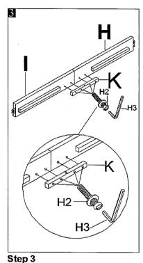
Attach wood bar "K" to the 2 rails "H" & "I". Using wrench (H3) to lock with bolts "H2".
