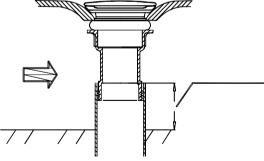
1. Insert the outlet pipe into the sewer pipe. If the outlet pipe is too short,Please connect it with a tube before inserting.
