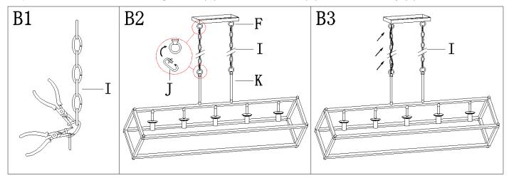
Step B1: By measuring, determine the correct number of links needed for proper hanging height. Using the chain pliers, disconnect and discard the unwanted part.
