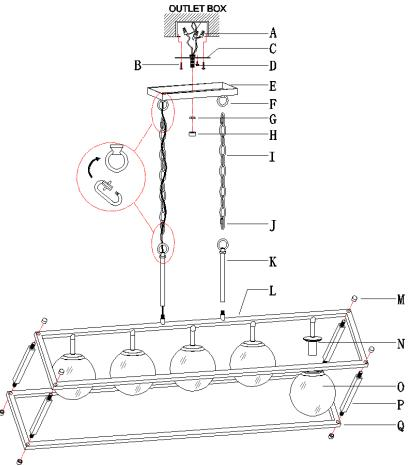
Step A1: Secure threaded pipes (P) onto lower frame (Q) and fixture body (L) with lock nuts (M).
