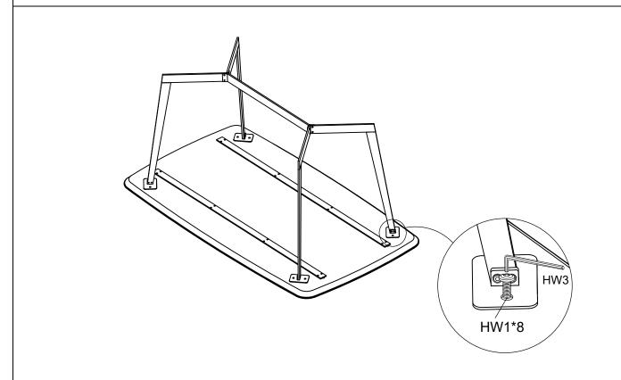
STEP2 assemble metal legs on body
