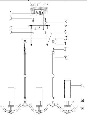
Step A1: According to your desired hanging height, choose and use the stems (K). Carefully thread the fixture wires through the stem (K), then screw the stem (K) onto the iron frame (N).
