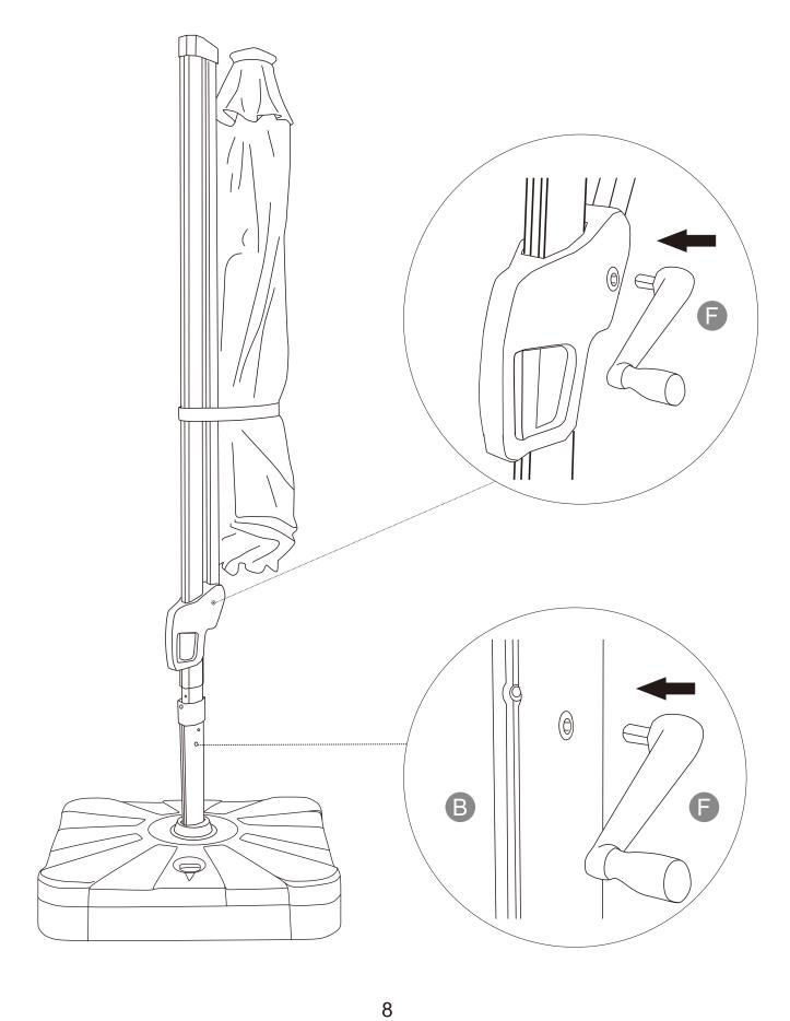
**Step 6**: To open the umbrella, squeeze the trigger and slide the glide handle up to a comfortable positon, then release the trigger to lock into place. Turn the Crank Handle (F) clockwise to fully open the canopy as pictured. Slide the glide handle up or down to achieve the desired tilting angle. Umbrella can be closed with the opposite operation.
