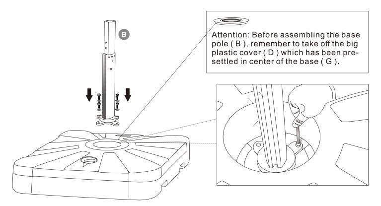
**Step 3**: Place the Plastic Cover ( D & C ) on the stands ( G ) through Base Pole ( B ) . Fix the Plastic Connector ( E ) on the Base Pole ( B ) . Make sure to line up the hole of connector with the lower hole on the Base Pole ( B ) .
