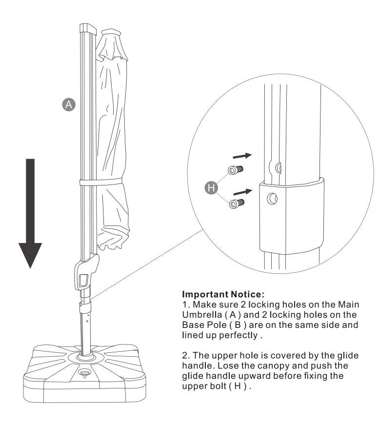
$\mbox{\bf Step 5}:$  Insert 2 Crank Handles ( F ) into the square holes on the glide handle and Base Pole ( B ) .
