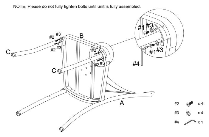
Step 3. Attach bottom frame (part D) to back panel (part A) and legs (part C) using bolts (part #2), washers (part #3) and allen wrench (part #4).
