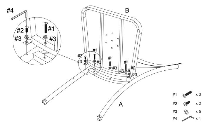
Step 2. Attach legs (part C) to seat panel (part B) using bolts (part #2), washers (part #3) and allen wrench (part #4).
