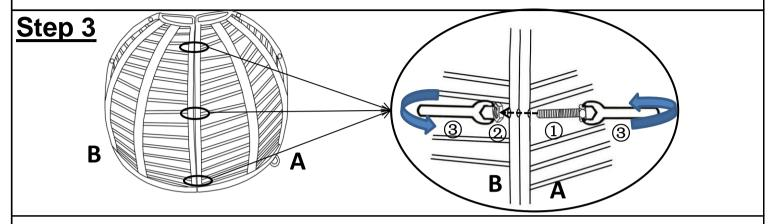
After finished above step 2, please connect Top(A) to Left Back(B), using the screw(1) and nut(2) with Spanner(3).
