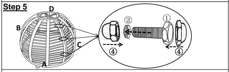
Attached Screw protector gap set(4) to all screw(2) and Nut(1) by hand.
