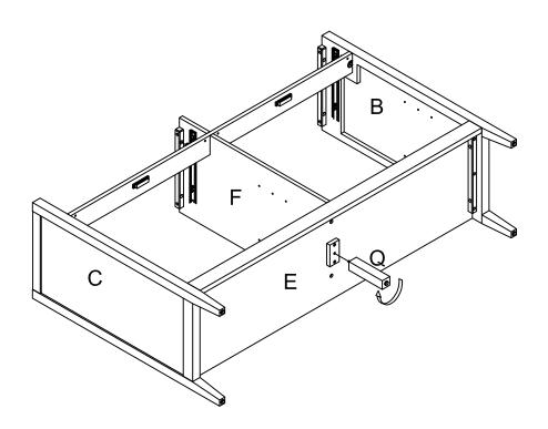
Step 7. Carefully turn unit upright. Attach top panel (part A) to assembled unit (parts B, C & F) using wood dowels (part #5), short bolts (part #1), spring washers (part #2), flat washers (part #3) and
