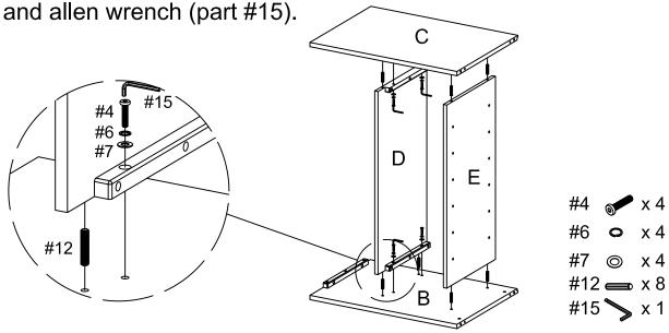
Step 6. Attach top panel (part A) to panels (parts B & C) using wood dowels (part #12), short bolts (part #4), spring washers (part #6), flat washers (part #7) and allen wrench (part #15).
