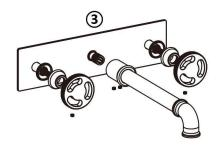
3. As shown in Figure 3 After finishing the wall decoration, Install the decorative sheet, decorative cover, spout and handle correctly.
