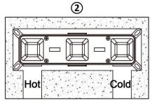
2. Install the concealed box on the wall, and connect the G1/2 hot and cold water supply pipe with the "Hot water" sign on the left (Figure 2). Note: Ensure that the center line of the valve body is perpendicular to the wall and the upper plane of the concealed box is horizontal. Keep the plastic shield on the valve body during installatio.
