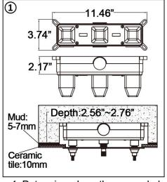
1. Determine where the concealed valve will be installed on the wall. Make a suitable hole in the wall (Figure 1).
