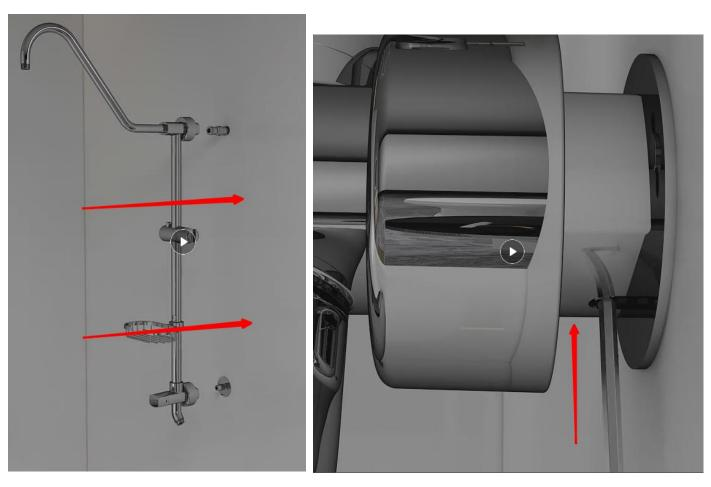
Step 9 Install other parts of the shower, taking care to check that the shims are placed inside.
