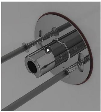
Step 8 Install the whole product on the wall, push the top and bottom two decorative covers outwards, use a hexagonal wrench to tighten the screws clockwise, and then push the decorative cover back toward the wall.
