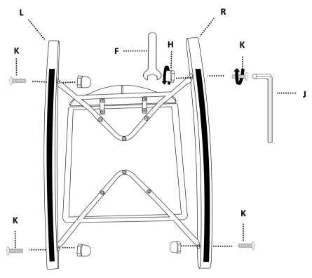
4.As shown in the figure, Do not tighten all the screws at once.
