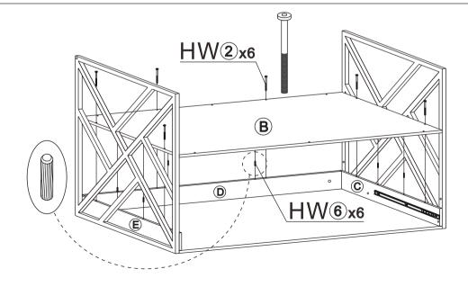
**STEP6:** Attach part ©, D, E to B using HW 6, insert HW 2 in pre-drilled holes and tighten them.
