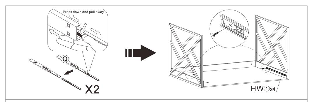
**STEP5:** Separate part (a) into two parts, attach the big part of (a) to part (c), (E) using HW(1).
