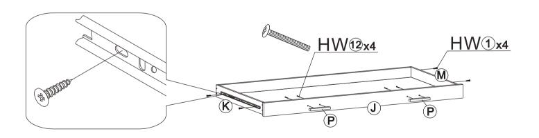
**STEP14:** Attach part Pto Jusing HW 2, attach the samll part of Qto part K, Musing HW 1.
