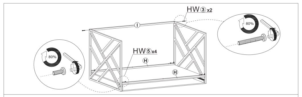
**STEP7:** Attach part ①to ⑥, ⑥ using HW ③, attach part ④to ⑥, ⑥ using HW ⑤, please make HW ③, HW ⑤ to be locked 80% only.
