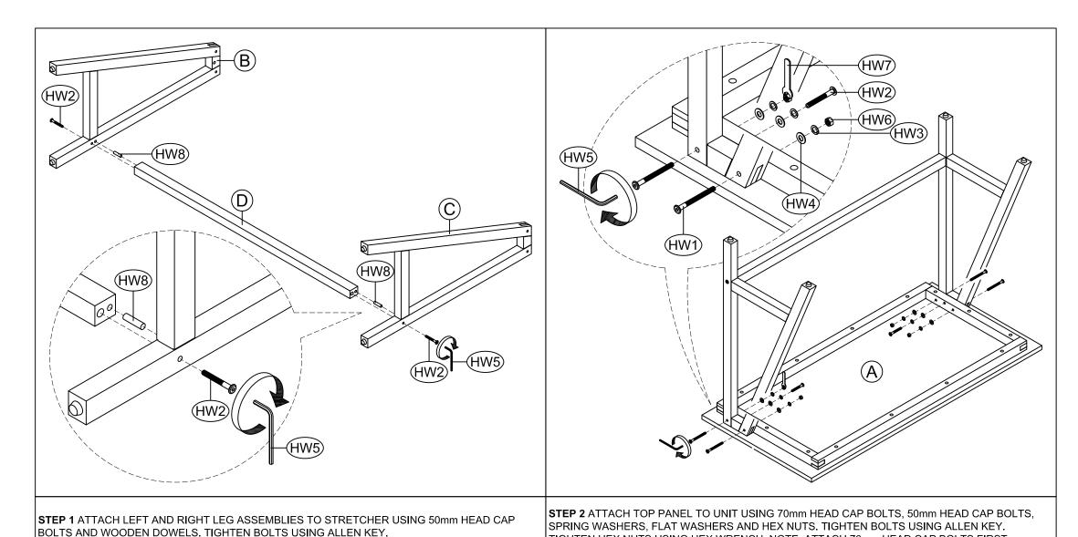
TIGHTEN HEX NUTS USING HEX WRENCH. NOTE: ATTACH 70mm HEAD CAP BOLTS FIRST.
