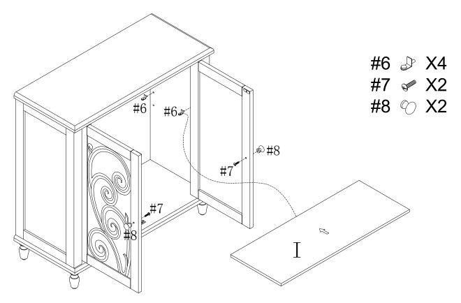
Insert the shelf holder(6)into the left panel(C)and right panel(D)horizontally. And place the shelf panel (I) in parallel. This is shown in the figure above. The handle(8) is fixed on the left door frame(E) and right door frame(F) and is locked with round head bolt(7).
