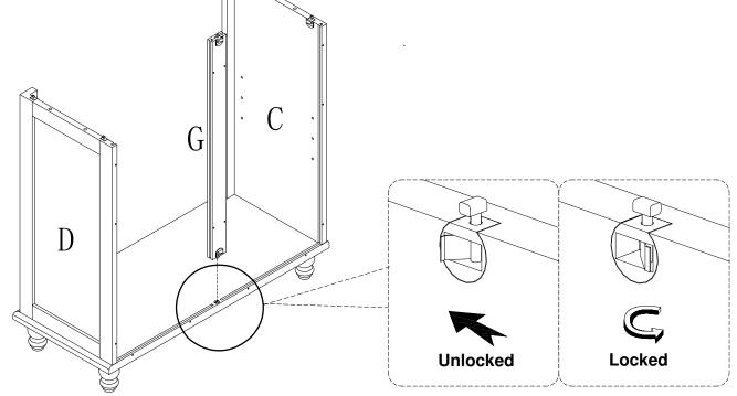
Buckle the back bar (G) into the bottom panel(B) as is shown in the figure.
