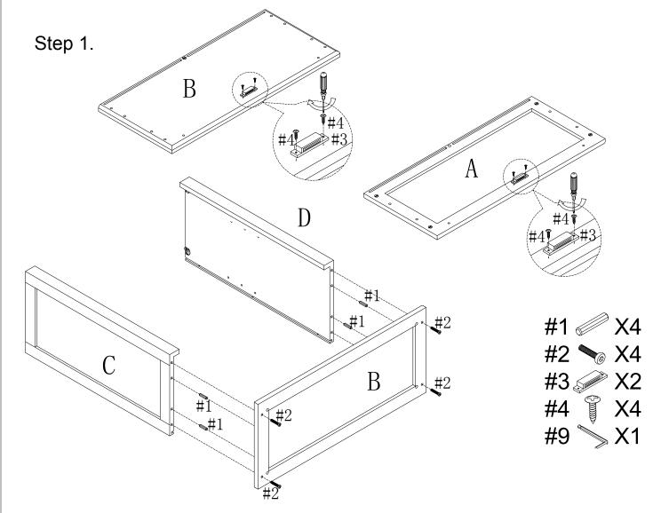
Attach door magnet(3) to top panel (A) and bottom panel(B) using screw(4). Insert wood dowel(1) to left panel(C) and right panel(D) and bolt(2) to bottom panel(B). and then lock with the allen key (9).
