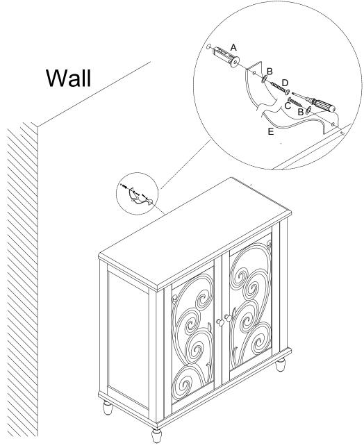
Drill 1 hole on the wall. Insert wall anchor(A)into the wall.
