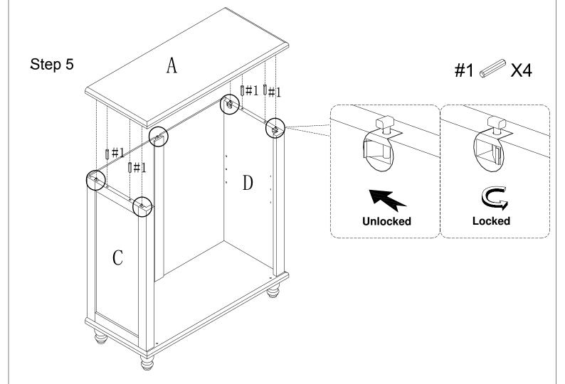
Insert wood dowel(1)to left panel(C) and right panel(D).
