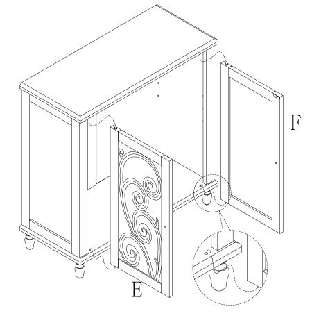
Slide door frames (E.F) as shown above, and align holes reserved in both top and bottom panel.(When holes are aligned, you usually can hear a slight clicking sound as they lock into place.)
