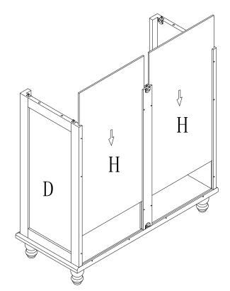
Slide back Panel(H)into grooves as per diagram.
