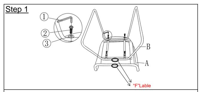
Note: Locate the sticker with the "F", and ensure this side is facing frontwards.
