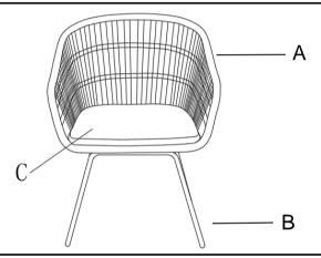
Put the Cushion (C) onto the Chair. Then tie the rope on the Cushion (C) to the Seat (B).
