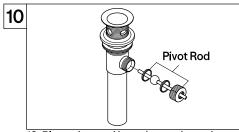
10. Place pivot rod into pivot rod opening. Slide pivot nut over pivot rod and thread it on the drain body. Tighten firmly.
