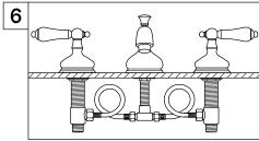
6. Attach flexible hoses to the outlet port of hot and cold valve assembly, you may need to loop the hoses as shown on graphic and be careful not to overtighten.
