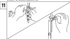
11. Guide the pivot rod through one of the holes on the lift rod strap and secure it with the spring clip. Then adjust the height of the lift rod by resetting the clevis screw. With lift rod in position on the faucet, insert lift rod through lift rod strap and secure with the clevis screw.
