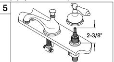
5. While holding from underneath sink, thread top lock nut from above, set height of stem at estimate 2-3/8" for KS1161\* group from the deck to the tip of the stem. Secure both top and bottom lock nuts, do not over tighten lock nut as this may cause undue stress on stem body and cause leaking, which may result in water damage. Thread escutcheon onto valve assembly and install the handle.
