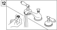
12. Remove the aerator, turn on the faucet. let water run for at least one minute, this will clear any debris left in the line, reinstall aerator.
