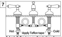
7. Apply Teflon tape on all male threading and install inlet supply lines (not included) to bottom inlet port of hot and cold valve assembly.
