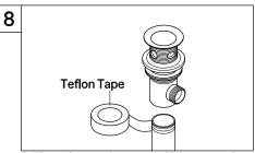
8. Thread mounting nut and bottom gasket onto drain body. Wrap top threaded end of the drain body with Teflon tape.
