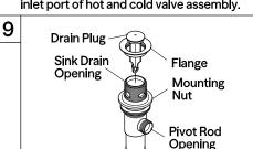
9. Apply silicone to bottom side of flange. Install flange body up through the drain opening, hold the drain flange body in position with pivot rod opening facing the back of sink and hand tighten the mounting nut. Be sure to clean excess silicone.
