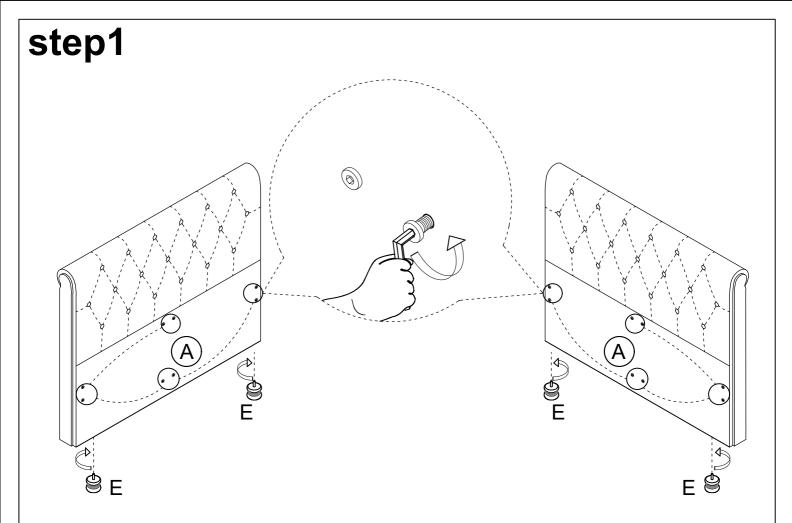
Loosen the pre locked screws.
