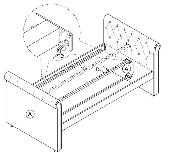
Put the part "D"on part "A",then tighten all the pre -locked screws.
