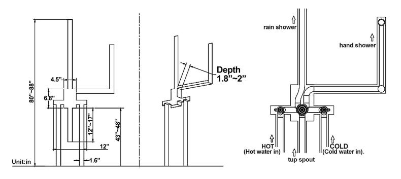
3. Fix the main body of the faucet with self-tapping screws (the main body must be flush with the wall).
