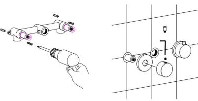
4. Install outlet pipe(Convovle Teflon tape round screw).
