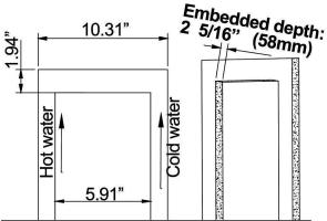
Note: depth of embedded box excavation thickness of tiles to be reserved.
