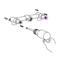
4. Install outlet pipe(Convovle Teflon tape round screw).
