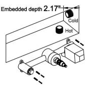
4. Use the hexagon key to install the switch handle and install the color button.
