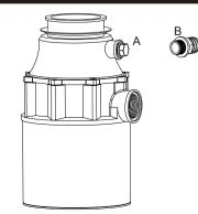
**NOTE:** If the dishwasher connection is made without removing the plug. the dishwasher may overflow. (Connections must comply with local plum bing codes.)
