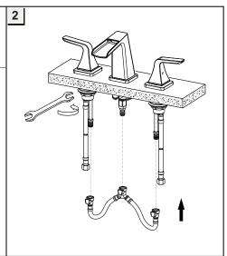
Use hand to screw up the locknut, then use install tool for fixing strengthen. And then connect the outlet hose as shown.
