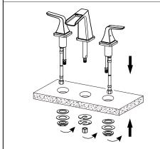
1. Please confirm the three holes on the basin are through holes as shown from the instructions before install. First, remove all fixing sets from the fixed group, and then put the body through the hole on the basin, assemble all fixing sets to the body.
