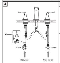
3. Connect the inlet hose as shown, take note of the "Red" & "Blue" index from the handle, "Red" for connecting to the valve for supply hot water, and "Blue" for connecting to the valve for supply cold water.
