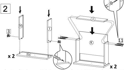
Combine Side Drawers ( H & I ) using Insert Cambolt (HW1) into Camlock (HW3), tighten Camlock (HW2) using screwdriver.
