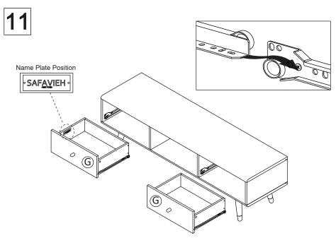
Use Wedge (HW12), Screw M 3.5 x15.5 (HW13) to tighten the back of media stand by using screwdriver. Use Back Panel Holder (HW20) and Screw M4 x 17 (HW19) to hold the Back Panel altogether.
