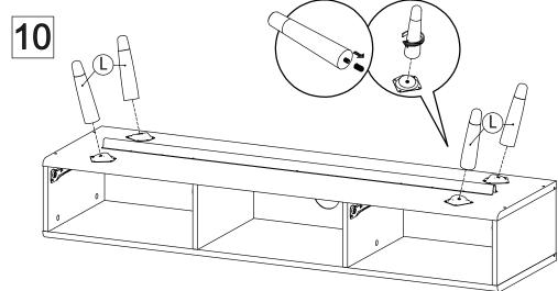
Place Anti Deflection Metal Bar (HW16), secure with screw M6x10,5 using screwdriver.
