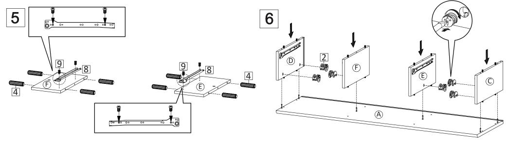
Insert Dowel Big (HW4) into Center Board Left (E) and Center Board Right (F). Continue with securing part of the metal runner (HW8) into position as the above image, using screw M6x10,5mm (HW9)
