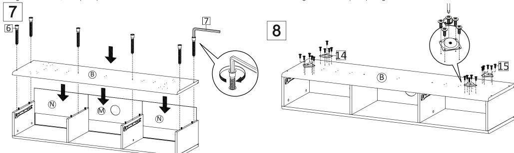
Insert Back Board 1 (N) into position at left and right.
