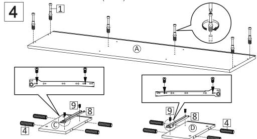
Insert Cambolt (HW1) into Top Board (A)
