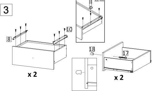
Bring the Drawer from Step 2 upside down, install the metal runner (HW8) into position as shown in picture, secure with screws M3.5x13 (HW10) Use Screw M 3.5x25 mm (HW17) to attach Handle (HW18) to the Front Drawer as above image.
