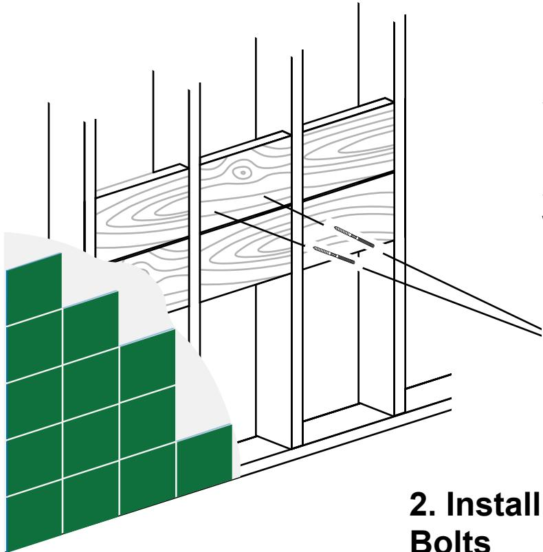
Locate studs in the wall. If the studs do not line up with the holes in the back of the sink, be sure to add sufficient wall supports behind the finished wall.
