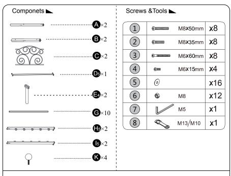
Check all the components & screws before assembly. Do not install in case part is missing, contact us to get. Send email with your question to support@vecelo.com. We will resend within 24 hours.
