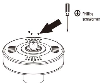
Overlap the ceiling bell and ceiling fan housing after aligning the holes.
