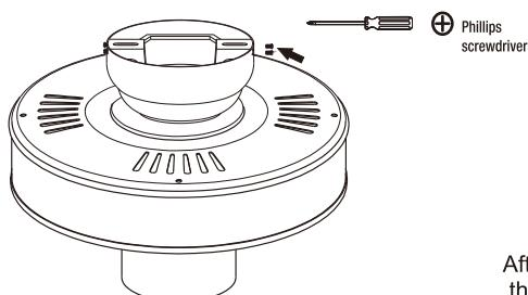
After the power cord is connected, arrange the power cord in order, then clip the keyhole of the bell into the screw on the hanger and lock it, then use the screwdriver to lock the other two screws.
