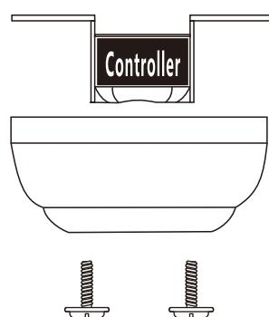
1: Remove the mounting bracket from the canopy by loosening the two canopy screws located in the L shaped slots.
