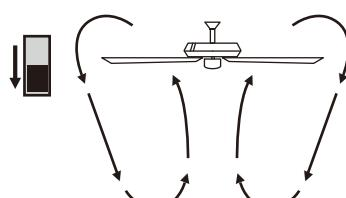
A.warm weather-(Forward) A Downward airflow creates a cooling effect. This allows you to set your air conditioner on a higher setting without affecting your comfort.
