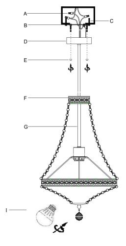
PLEASUE USE TYPE"A" BULB MAX 60-WATT OR CFL MAX 13 WATT OR LED BULB MAX 9-WATT THERE IS 1\*9W LED BULB IN THE BOX.
