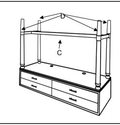
legs, Screw four feet thourgh bottom board to connect with legs.
