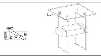
STEP 4: Carefully place table base with the STEP 5: Carefully insert the glass table top onto the empty side of the middle board skywards, and glass legs by aligning into the slots of glass clips. attach the EVA Foam Mat (HW6) on the four Tighten the side screws of the glass clips with Allen Key
