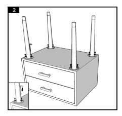
Step 2: Press the leg into bottom of cabinet and tighten allen bolt onto 3 holes of cabinet by Allen key
