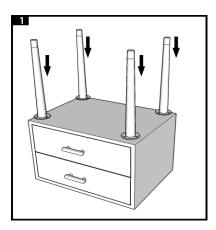
Step 1: Put cabinet on a smooth and soft surface. Then put the leg of the cabinet in the right place
