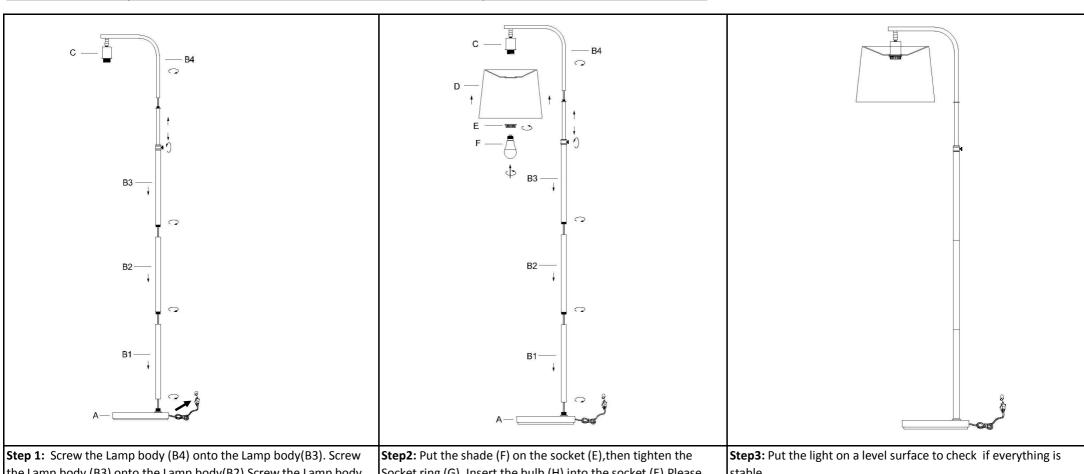
the Lamp body (B3) onto the Lamp body(B2). Screw the Lamp body (B2) onto the Lamp body(B1).
