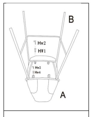
Align the base (B) onto the bottom of seat(A) as pictured. Use allen key "HW2" to lock the 2 screws "HW1".
