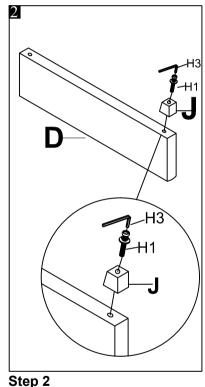
Attach wood legs "J" with footboard "D". Using Allen key (H3) to lock with bolts "H1".
