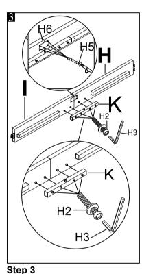
Attach wood bar "K" to the 2 rails "H" & "I". Using Allen key (H3) to lock with bolts "H2".
