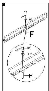
Attach support legs "F" to wood bar "K" .Using Allen key (H3) to lock with bolts "H2".
