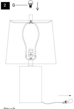
Step2 Insert the bulb(G) into the socket(C).
