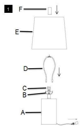
Step 1 Insert the Harp (D) into the Saddle (B). Put the shade(E) on the Harp(D), then tighten the Finial (F)into the Harp (D)
