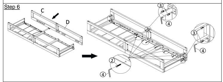
With assistance from your adult partner(s), attach the assembled part in Step 2 - the Left Backrest Base Panel (C) and the Left Seat Base Panel (D) to the assembled part in Step 5 using Bolts (2), Screws (3) and the Allen Wrench (4) as shown in the pictures above.
