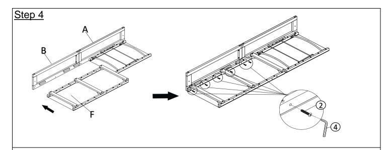
With assistance from your adult partner(s), attach the Seat Panel (F) to the assembled parts in Step 3 using Bolts (2) and the Allen Wrench (4) as shown in the pictures above.
