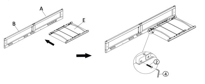
With assistance from your adult partner(s), attach the Backrest Panel (E) to the assembled parts in Step 2 - the Right Backrest Base Panel (A) and the Right Seat Base Panel (B) using Bolts (2) and the Allen Wrench (4) as shown in the pictures above.
