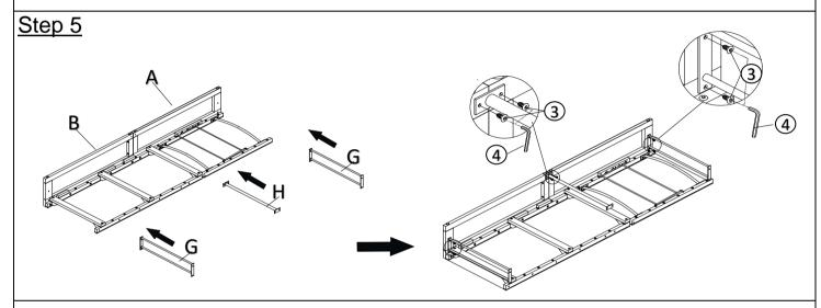
With assistance from your adult partner(s), attach the First Support bar (G) and the Second Support Bar (H) to the assembled parts in Step 4 using Screws ( $\mathfrak{J}$ ) and the Allen Wrench ( $\mathfrak{J}$ ) as shown in the pictures above. **Do not fully tighten the Screws at this time.**
