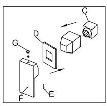
3. Remove the prastic cover (D) and then put the base through the cartridge cover (C), use Alleny key (E) and the hexagon socket screw to assemble the handle (F) to the body, and then put on the decorative button (G).
