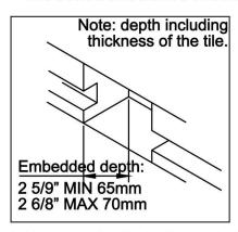
1. Holes size for the built in control valve: 3.94"(100mm)X3.94"(100mm) X2.56"~2.76"(65~70mm), the depth between the bottom of the control valve to the tile surfaceis 2.56"~2.76" (65~70mm).
