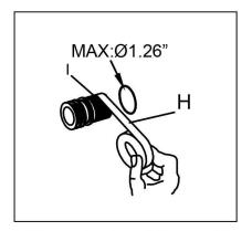
4. Wrap nylon tape (H) around the screw thread at the end of thread pipe, and then tighten the thread pipe (I) to the water pipe.
