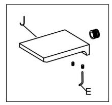
5. Fix the spout (J) to the position block and the thread pipe, and then use the Allen key (E) to tight the spout with the thread pipe.
