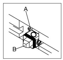
2. Use the tape on pipe threads, connected to the main body (A) cold and hot as required inlet pipe and outlet pipe, checking the leakage before fixing the main body in the embedded hole (keep the horizontal and vertical). Do not remove the protective plastic cover (B) during assembly to ensure watertightness and then landfill.
