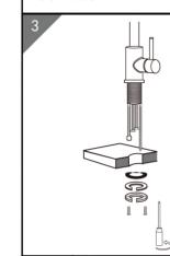
Install the faucet body into the hole. Ensure the rubber gasket is just below the bottom of the sink or countertop, and reassemble the parts in the order shown.
