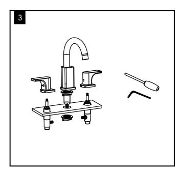
3. Put the spout and handles through the holes on the bathtub, adjust them to the proper direction and tighten them with the screws. The direction of the handles shown in the picture is Turn On.
