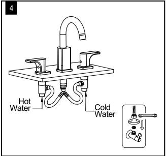
4. Connect the hose to the spout and handles firstly, and then connect the inlet pipes, Red hot Blue cold, connect the other end of the inlet pipes to the angle valve.
